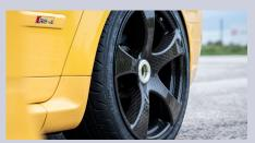
CompPair and Kling Technology have manufactured a healable carbon rim to offer high quality performance to the automotive industry, allowing multiple repairs to extend the lifetime and quality of a wheel rim.
